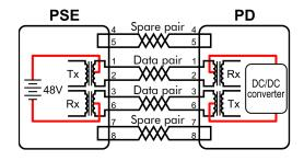
The data and the power supply pass in the same Ethernet cable, so there is only one cable to be pulled per connected device. Therefore, compared to an external power supply, the amount of connectors and adapters is reduced..
